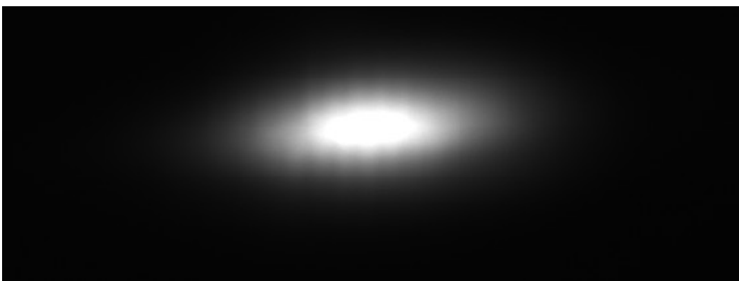
FIGURE 4.31: Captured atoms in the magneto-optical trap. The atoms scatter the light of the laser beams and this can be used for fluorescence imaging. The 1 : 1 telescope projects the magneto-optical trap to a charged-coupled device (CCD) camera. The new apparatus in the laboratory container has been operated with argon ( ^{40}\text{Ar} ) and krypton ( ^{84}\text{Kr} ). The image shows the first magneto-optical trap with ^{84}\text{Kr} in the container.
