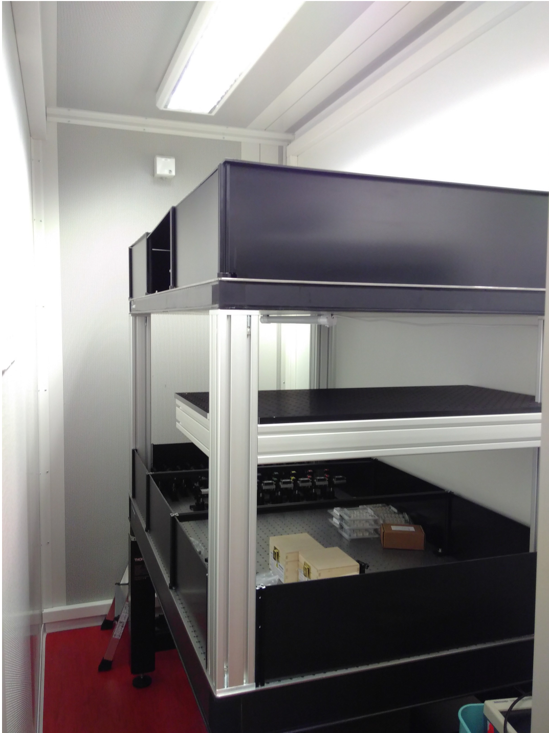
FIGURE 4.7: Photo of the two layer optical table. The laser setup and light amplification is built on the top layer while the bottom layer houses the frequency shifting. An intermediate layer was added to store the fiber-coupled closed spectroscopy cells and optics for offset-locking.
